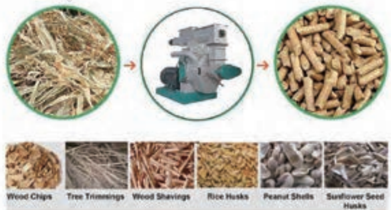
Wood pellet fuel processing equipment
